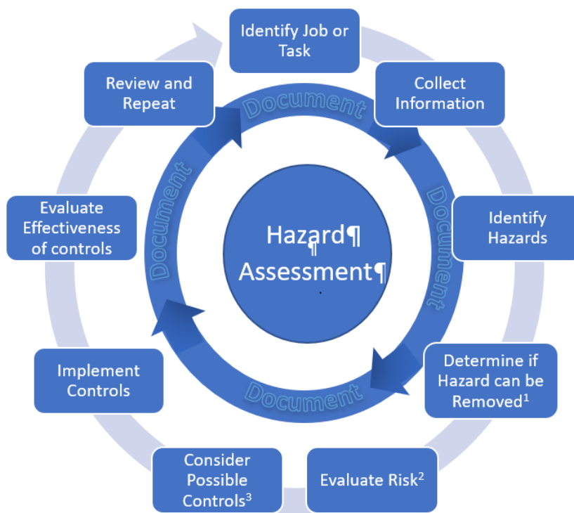
Figure 1: Hazard Assessment Process
